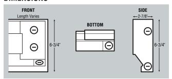
All knockouts are 7/8" diameter for 1/2" conduit
