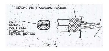
7. Wrap the sealing putty around both heaters. Use the whole length of sealant provided. Mold the sealant around the heaters so that it fills in the spaces between the heaters and assumes the shape of the heater jacket. Mold the sealant on the outside of the heaters so it is slightly larger than the heaters' outer jacket (see figure 6).
