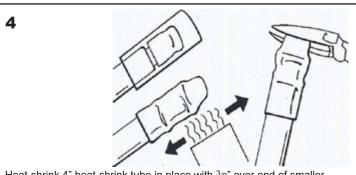
Heat-shrink 4" heat-shrink tube in place with \$\frac{3}{18}\] over end of smaller heat-shrink tube. Remove heat, resqueeze at end of smaller heat-shrink tube, then squeeze at end of outer heat-shrink tube. Hold for 10 to15 seconds.
