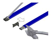
Apply RTV sealant into end cap and also over 1 inch of the end of heater.
