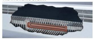
The electric heating element is partially submerged in an inert heat transfer fluid totally sealed in a large 7/8" diameter copper tube spanning the length of the heater. This thermal mass transfers heat evenly across the entire length of the heater. The PLF series provides uniform warmth with longer heat retention and minimal temperature variation.
