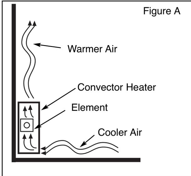
In convective heaters the heated air rises (exits) at or near the top of the heater and through a process called “chimney effect” draws cooler air into the heater at or near the bottom of the convector. This air is heated, rises and exits at or near the top of the heater in a continuing cycle (Figure A).
