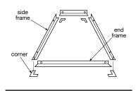
Frame construction for recessed panels
