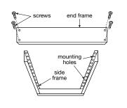
Frame construction for surface mount panels
