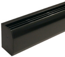
Bottom inlet unit is only 2 5/8 in. wide by 4 in. tall. Can be mounted to wall (2 in. above floor) or in front of window mounted on pedestals.
