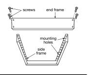
Frame construction for surface mount panels
