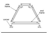
Frame construction for recessed panels
