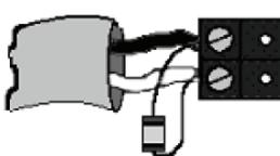
Figure 9: Terminating Resistor Detail
