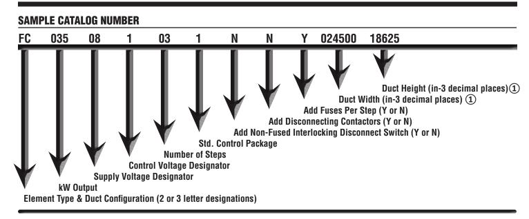
1 - On standard heaters width (W) must not exceed 144" and height must not exceed 96". Consult factory for larger heaters.
