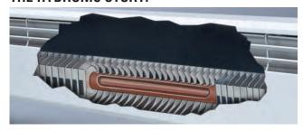
The electric heating element is partially submerged in an inert heat transfer fluid totally sealed in a large 7/8" diameter copper tube spanning the length of the heater. This thermal mass transfers heat evenly across the entire length of the heater. The FHP series provides uniform warmth with longer heat retention and minimal temperature variation.
