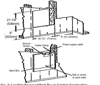
Fig. 2: Locating Recessed Back Box in Existing Construction
