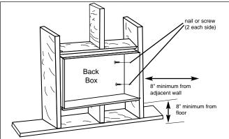
Fig. 1: Locating Recessed Back Box in New Construction
