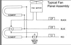
Wiring diagram for fan panels used on 208V, 240V, 277V Q Series
