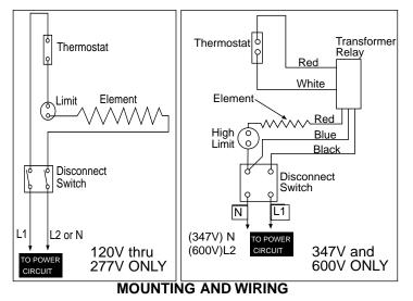
**NOTE:** Electrical wiring is to be sized in accordance with National Electric Code and local codes using at least 75°C type RH, THW or equivalent insulated wire. See chart located on page 3 for amp. loads.
